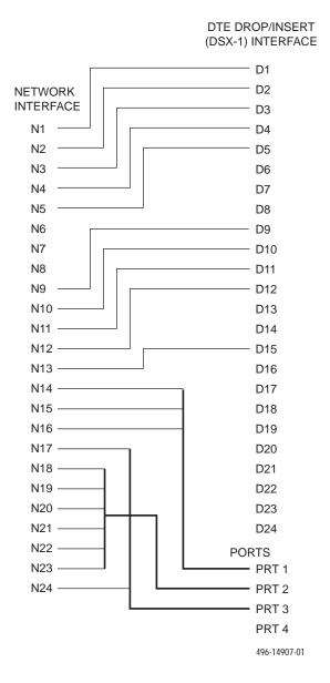
Figure 3-6. Example of Channel Allocation
